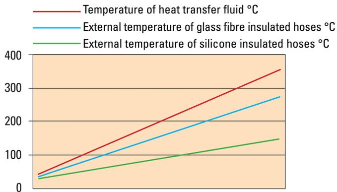
Hoses are made from stainless steel, are flexible, and suitable for use up to 400 °C. End connections are plasma welded. Supplied with either glass fibre or silicone insulation.
