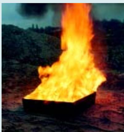
Trough with mesh. Filled with 3 x 2 l volumes of burning n-heptane. Flame extinguished in 2 - 5 sec for each 2 l volume.
