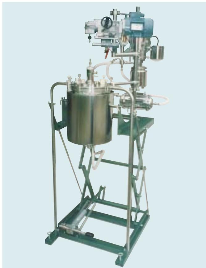
10 litre insulated vacuum vessel with lifting stage and thermostat.
