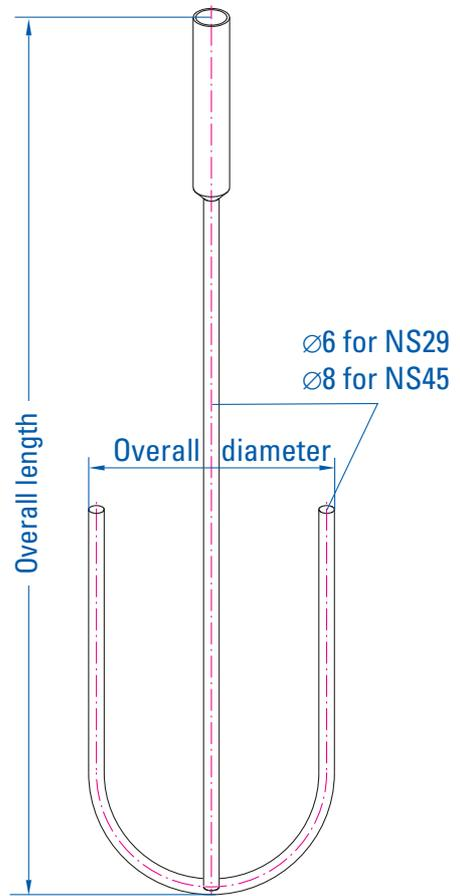
Anchor stirrers for Quickfit flasks
