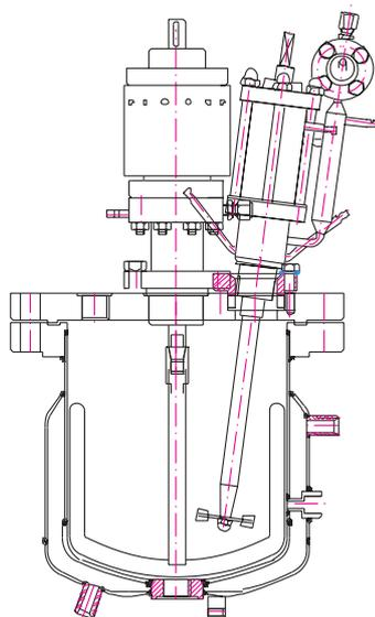
The drawing shows a 5 litre vessel with a centrally mounted 16 Nm magnetic stirrerhead and a sloping mechanically sealed stirrerhead to one side.
