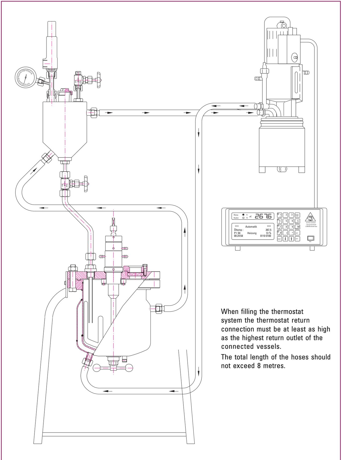
When filling the thermostat system the thermostat return connection must be at least as high as the highest return outlet of the connected vessels.
