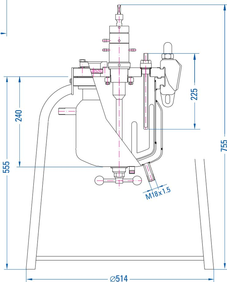
5 litre vessel with stirrerhead 10312.00 shown
