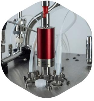
A manometer, overpressure protection and pressure relief valve are standard equipment.
